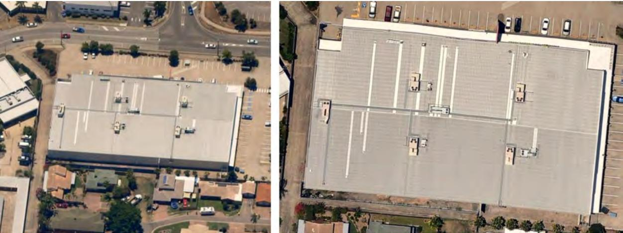
The site itself appears to be a large low pitched roof, with aged (& stained) zincalume steel sheeting. The roof area is approximately 3,900m<sup>2</sup> & would absorb extreme solar radiation exposure.
